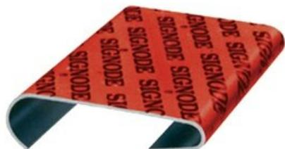
Signode 117 HDG OF Open-Flange seals are specifically designed for use with a N-1444-5LSH pneumatic sealer on 32mm Magnus steel strapping. Open-Flange seals are the heavy duty version of Snap-On seals. These seals are placed over the overlapping strap ends either before or after tensioning the strapping, eliminating pre-threading and increase productivity.
