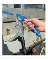
On the other side of the semi, tension the strap using the awning tightener.
