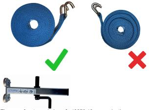
The use of a strap winder ref : 48879 12 can make the process easier
